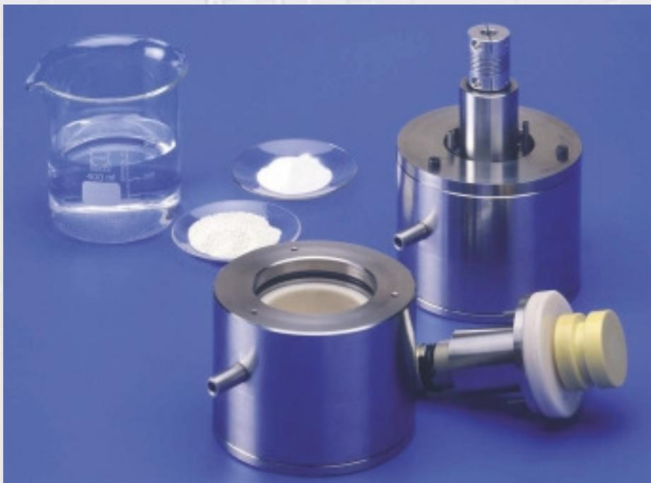
Fig. 1: Miniature bead mill for the laboratory. The rotor, cooled grinding basket and lid are made of ceramics, thus avoiding any contact of the grinding stock with metal. (Works photo Friatec AG Division Frialit-Degussit)
