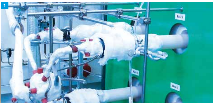
1 Tubes made of DEGUSSIT AL23 with analytic systems installed
