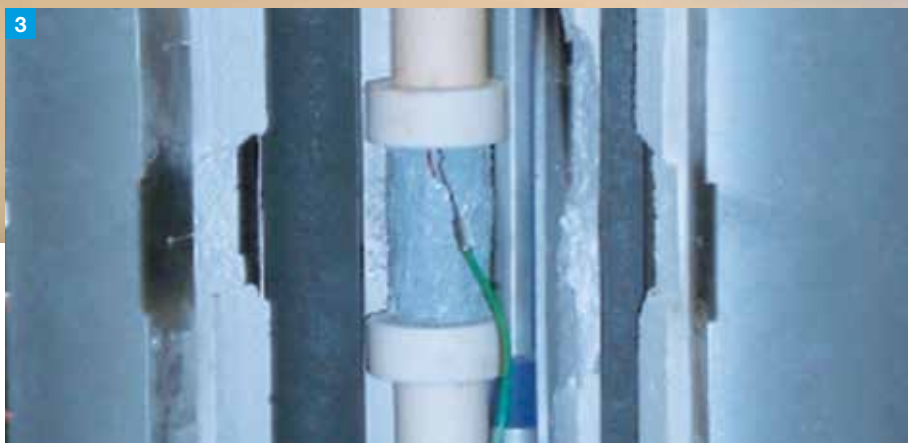
3-4 Components made of DEGUSSIT AL23 under thermal and mechanical stress
