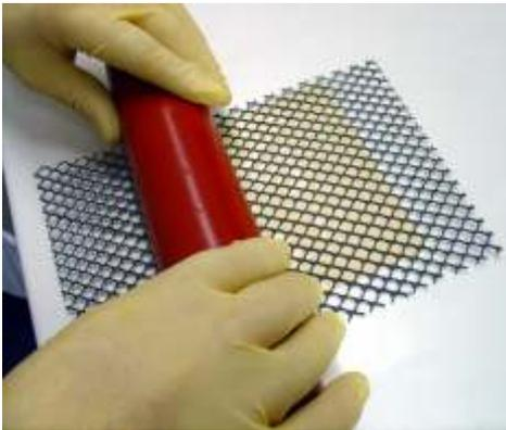
During manual embossing, uniform pressure is exerted with the aid of a roller.
